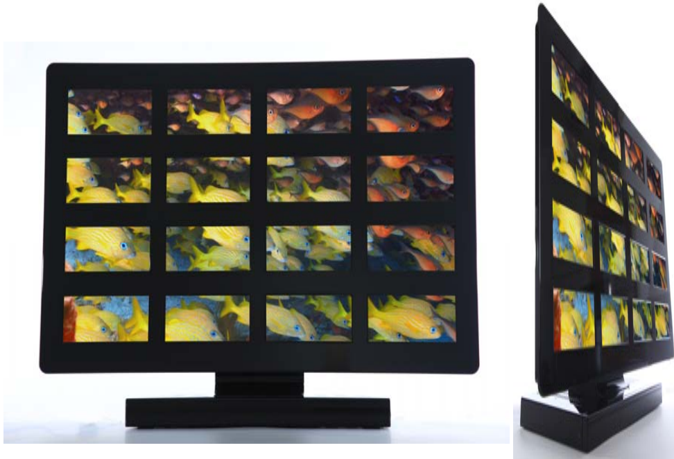
4.4" AMOLED Segment of 40" HDTV Printed solution-processed display
