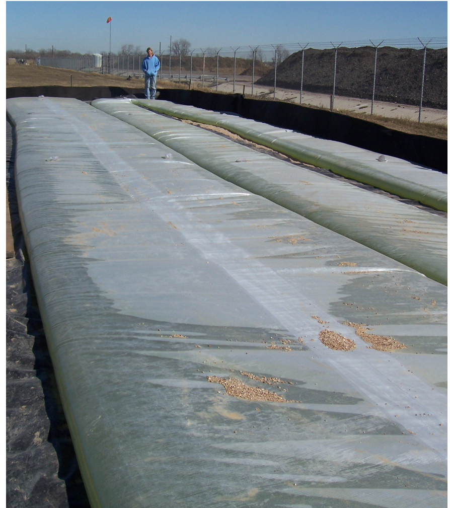
25,000 L Boomer™ production scale algae greenhouse (left)
