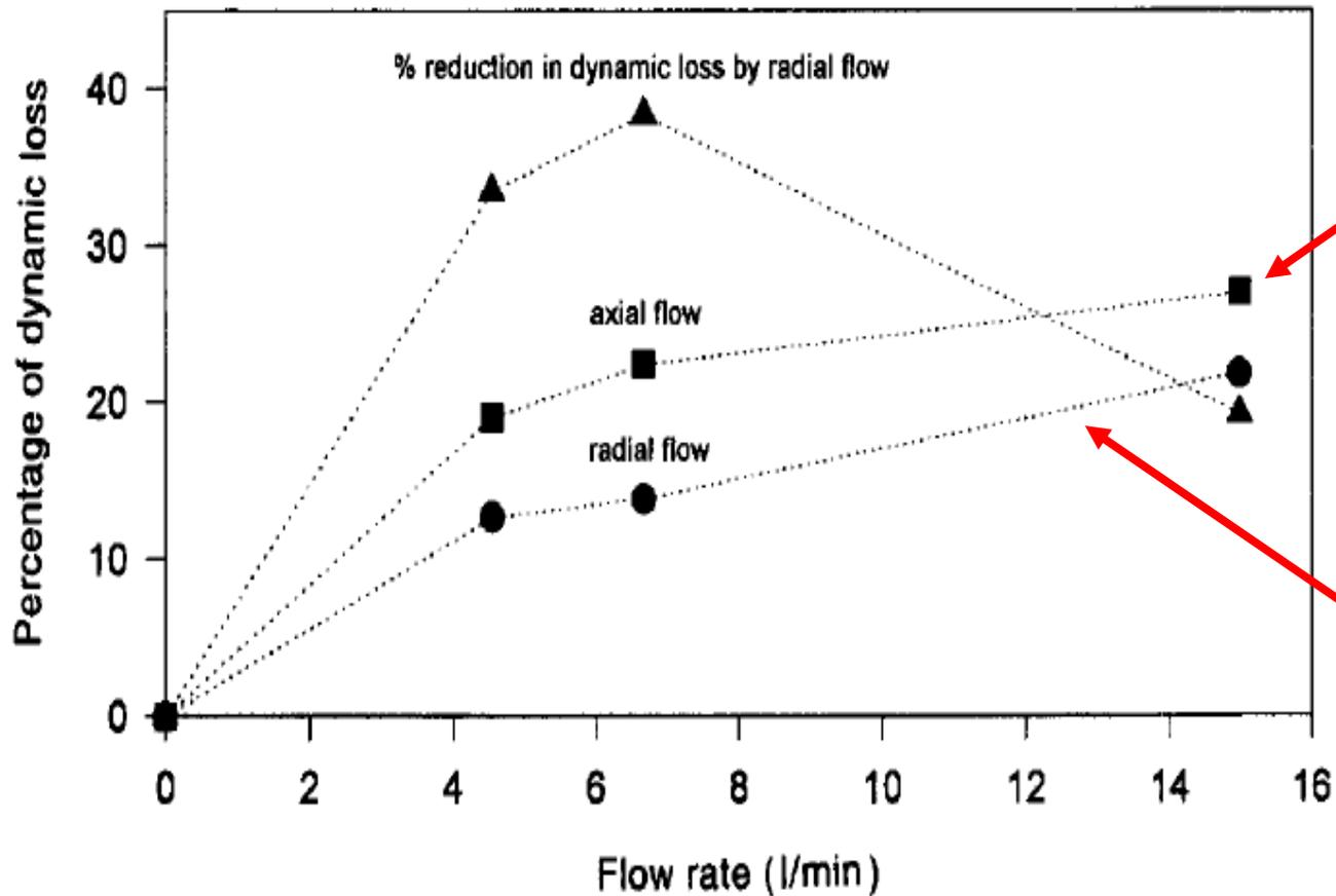
Fig. 12. Experimental data for the effect of flow direction during discharge of ANG cylinders.
